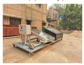
Solar-biomass hybrid dryer with thermal energy storage at TERI, New Delhi
